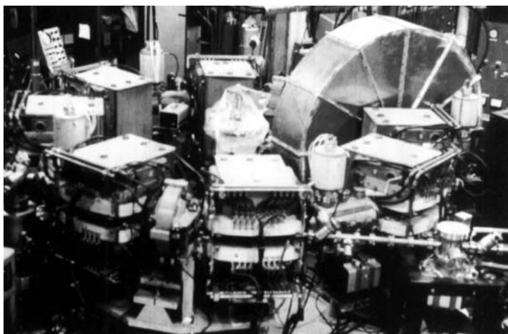
Figure 2. Tantalus in the early 1970s. Outside, the accelerator vault was shaped from a preexisting structure. Inside, the ring diameter was barely 3 meters and the beam half-life no longer than two hours.
