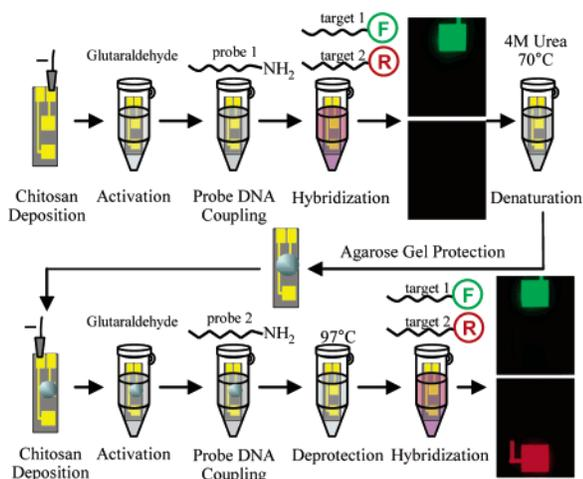
**Figure 4.** Sequential assembly of functional ssDNAs as shown by postassembly hybridization. The target DNA solution contains two target DNAs (fluorescein-labeled target 1 and Texas Red labeled target 2).
