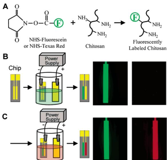
**Figure 1.** Sequential deposition of chitosan onto patterned surfaces. (A) Fluorescent labeling of chitosan with NHS-fluorescein or NHS-Texas Red. (B) Deposition of fluorescein-labeled chitosan. (C) Deposition of Texas Red labeled chitosan.
