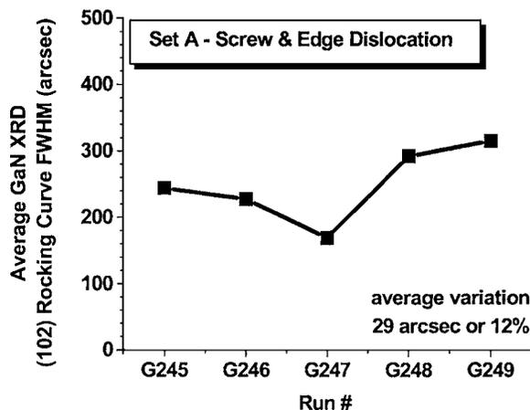
FIG. 6. Run-to-run variation in GaN epilayer crystal quality as measured by postprocess XRD shows average variation of 29 arcsec or 11%–12% for set A runs. The distortion of the (002) peak is indicative of screw dislocations, whereas that of the (102) peak is known to arise from both screw and edge dislocations.
