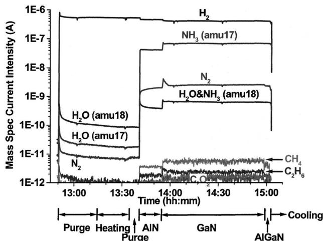
FIG. 4. *In situ* gas phase chemical signals from mass spectrometry, indicative of the dynamic gas composition downstream of the reactor as a function of process steps. The mass spectrometry current signals were acquired in real time through the entire HEMT growth process. Shown here is an example taken from run G262, for which the equipment configurations and process conditions are described in Table III.
