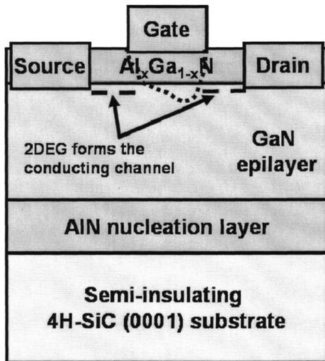
FIG. 1. Schematic representation of a HEMT based on AlGaIn/GaN/AlN/SiC heterostructure as grown by the MOCVD processes discussed in this article. Not drawn to scale.
