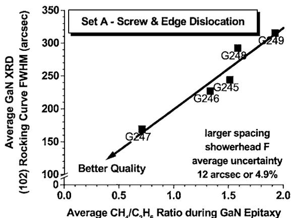
FIG. 7. Real-time prediction of GaN epilayer crystal quality during growth based on *in situ* measurement of methane/ethane byproducts ratio by mass spectrometry for set A runs. The metrology models show accuracies on the order of 5.1% average uncertainty for (002) peak and 4.9% for (102) peak, respectively. In general, narrower XRD rocking curve peaks represent better crystal quality, so in this case, it is apparent that smaller methane/ethane ratio is preferred for better GaN crystal quality.
