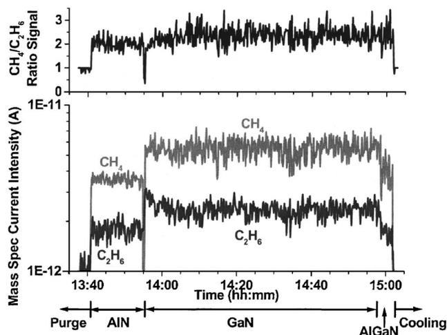
FIG. 5. *In situ* gas phase chemical signals from mass spectrometry, indicative of the dynamic gas composition downstream of the reactor as a function of process steps. Shown here are the reaction byproducts methane (at 13 amu) and ethane (at 26 amu) through the AlN, GaN, and AlGaN layer growth steps along with the corresponding methane/ethane ratio metric derived in real time. This example is taken from run G262, the same run as in Fig. 4.
