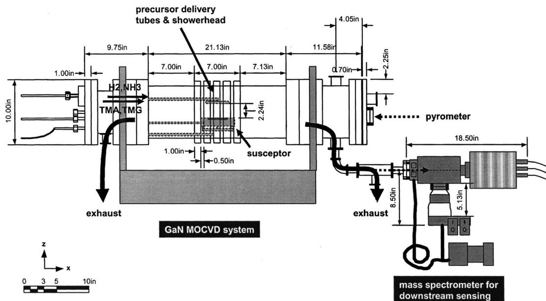
FIG. 3. Schematic representation of the 200 amu *in situ* quadrupole mass spectrometer gas sampling system (Inficon CPM™) attached to the downstream of the quartz wall reactor system for the GaN-based MOCVD processes discussed in this article.
