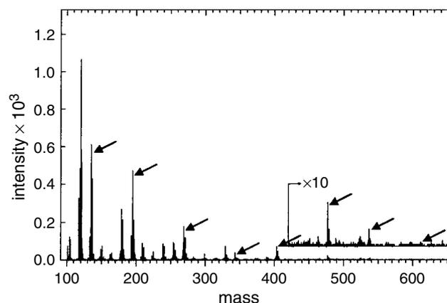
**Figure 4.** Negative static SIMS spectrum of sample 4-low-SiOH (175 °C, 1h).
