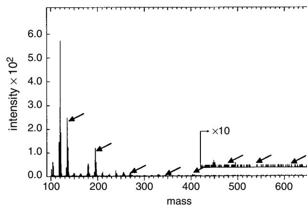
**Figure 5.** Negative static SIMS spectrum of sample 8-low-SiOH (450 °C, 2h).
