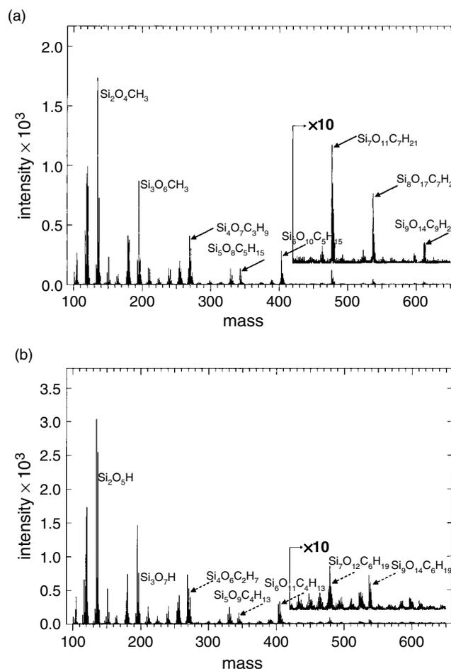
**Figure 1.** Negative static SIMS spectra: (a) sample 1-low-SiOH; (b) sample 1-high-SiOH.
