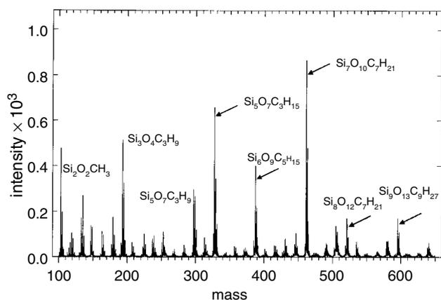
**Figure 2.** Positive static SIMS spectrum of sample 1-low-SiOH.
