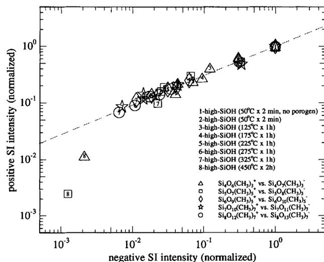
**Figure 6.** Intensity plot of key positive and negative species. Signals are normalized to species intensity as measured in sample 1-high-SiOH.
