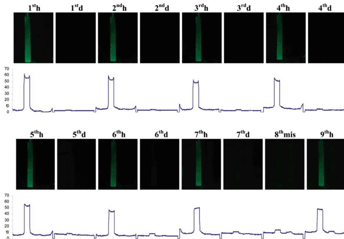
Figure 4. Repeated hybridization/denaturation of fluorescently labeled target DNA to surface probe DNA tethered to chip. "h" and "d" denote hybridization and denaturation, respectively. "8<sup>th</sup>mis" denotes eighth hybridization using 2.5  $\mu\text{M}$  mismatched target DNA. Final hybridization was performed using matched target DNA after 8<sup>th</sup> hybridization.
