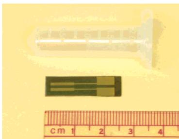
Figure 1. Nucleic acid hybridization chip composed of two gold patterns on a silicon nitride surface. Each chip fits within a 2-mL microcentrifuge tube.
