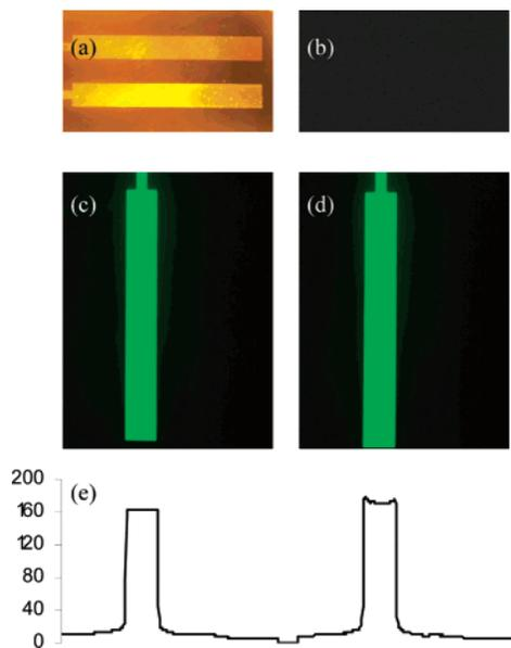
Figure 2. Assembly of ssDNA onto templated chitosan. (a) Bright-field image of gold patterns. (b) Fluorescence image of the chip after glutaraldehyde activation. (c) Fluorescence image of the chip after ssDNA assembly and brief buffer wash. (d) Fluorescence image of the chip after extensive urea wash. (e) Quantified fluorescence profile of (c) and (d), obtained by using Scion image analysis software.
