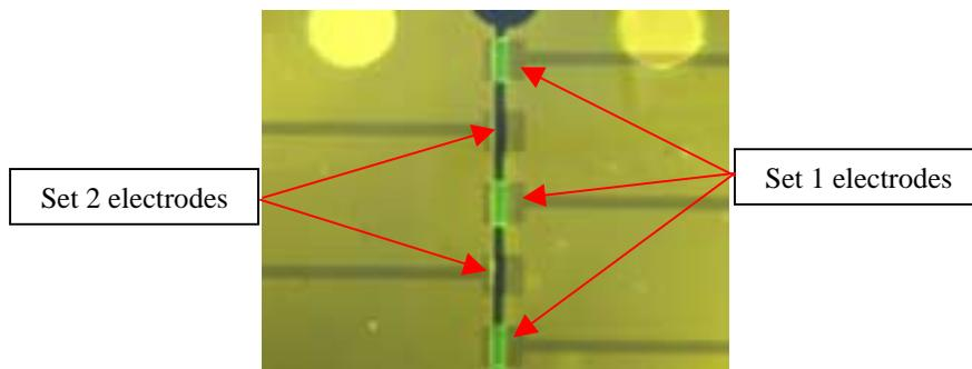
**Figure 9.** Bio-functionalization of the device. Model protein (GFP, green fluorescent protein) was coupled to chitosan (on set 1 electrodes) that had been templated onto the microfluidic channels. Standard glutaraldehyde-based chemistry was used to activate chitosan surfaces for subsequent protein coupling.
