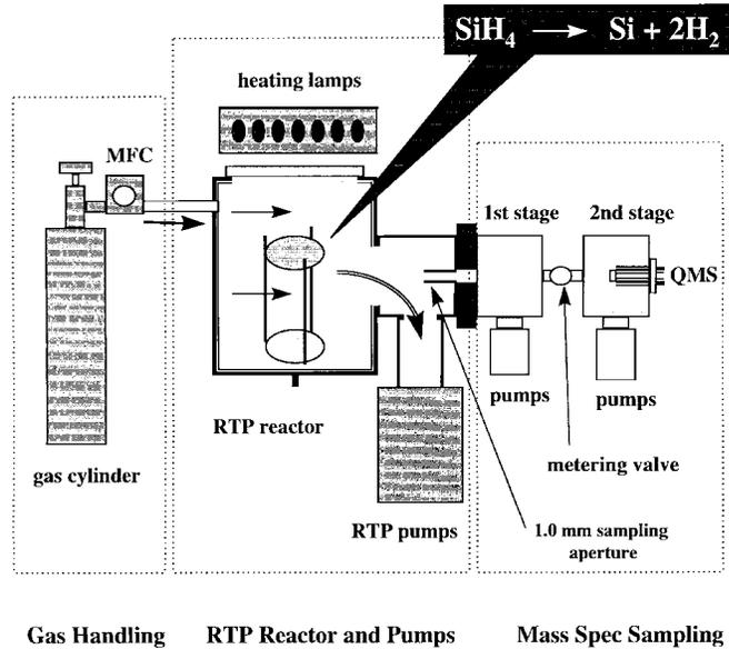
Fig. 1. Schematic representation of RTCVD module including gas handling, RTCVD reactor and pumping, and two-stage differentially pumped mass spectrometer system. The wafer is shown at the center of the reactor, where the silane decomposition reaction leads to Si film deposition.
