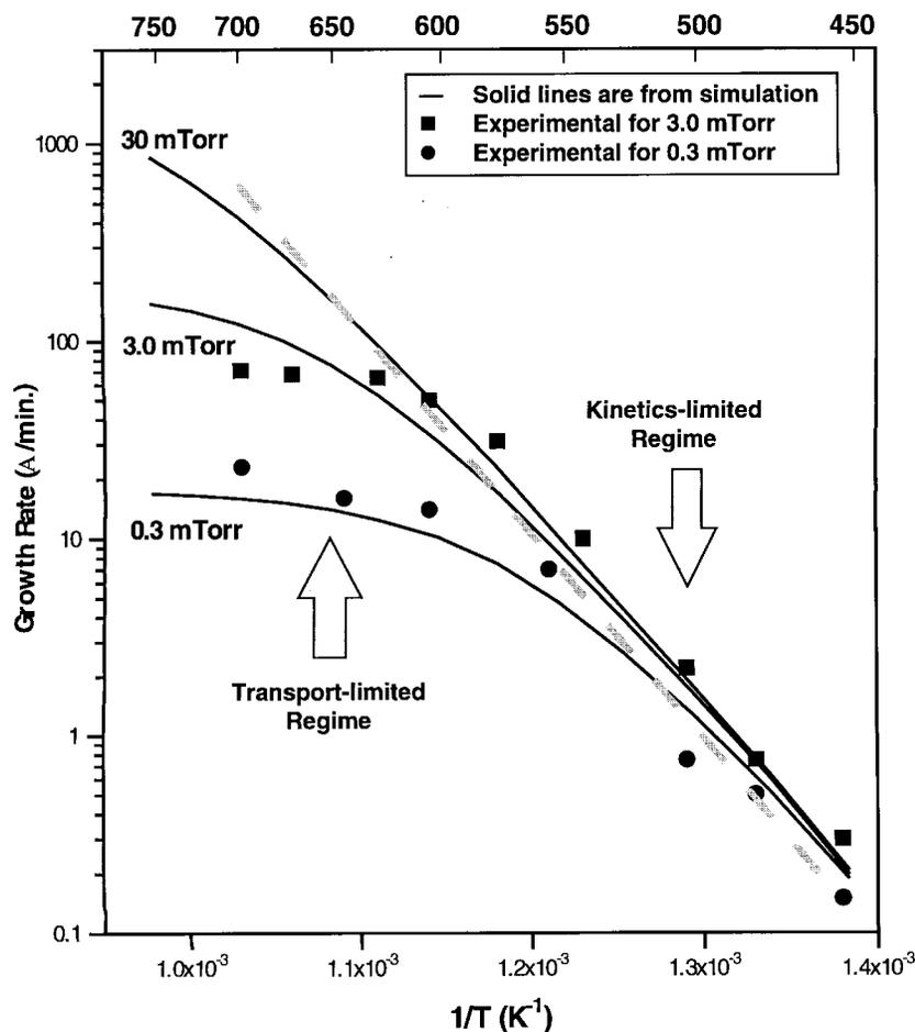
Fig. 4. Arrhenius plots of simulated polysilicon growth rate (as a function of  $1/T(K)$ ) at various  $\text{SiH}_4$  partial pressures. The transition from the surface reaction limited regime to the transport-limited regime is clearly observed from our simulation and is consistent with experimental results [13].
