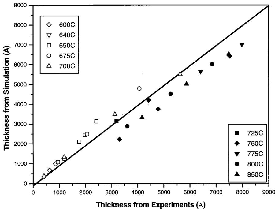
Fig. 7. Correlation plot of simulated and experimental film thickness for 27 deposition processes of polySi from  $\text{SiH}_4$ .
