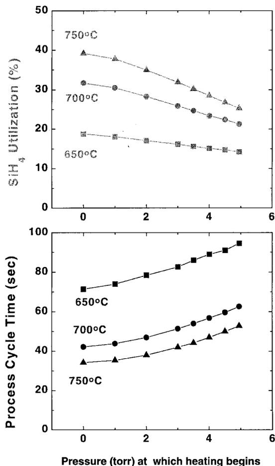
Fig. 9. Effect of process timing and process temperature on materials utilization efficiency (top panel) and process cycle time (bottom panel).
