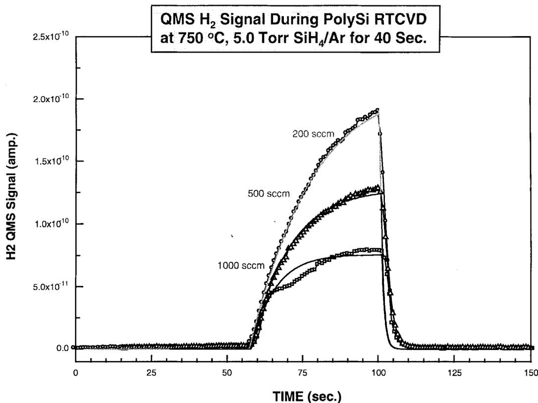
Fig. 6. Comparison of H<sub>2</sub> QMS signal during a deposition process for three different gas flow rates (200 sccm, 500 sccm, and 1000 sccm). The solid lines are from simulation and the data points are experimental measurements.
