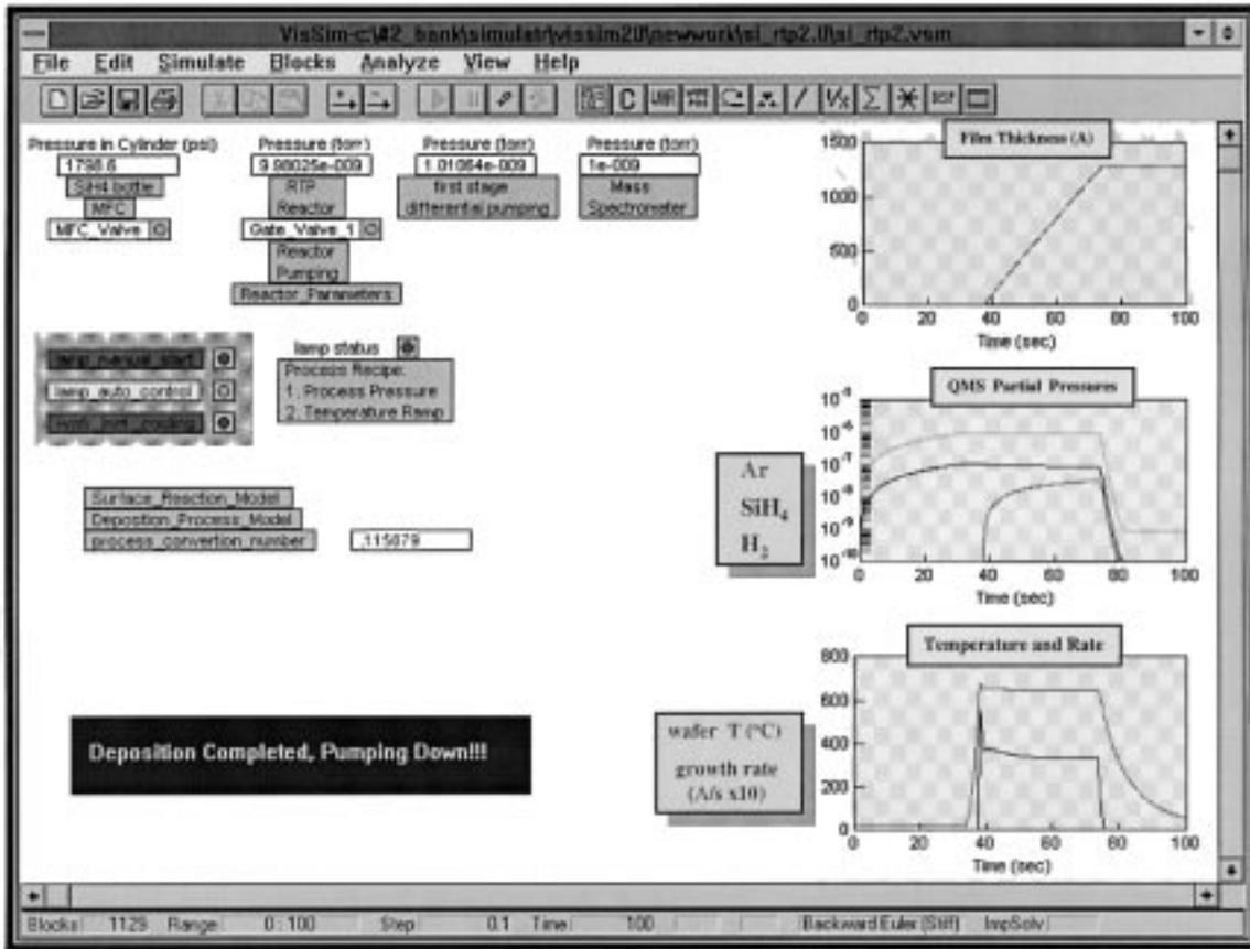
Fig. 3. Windows view of the RTCVD simulator. From top to bottom on the left-hand side of the window are the equipment simulator, the process recipe and control simulator, the deposition kinetics simulator, and a display panel for overall process status. The three plots on the right-hand side are simulation outputs for film thickness (top), QMS partial pressure signals (middle), and wafer temperature and growth rate (bottom).
