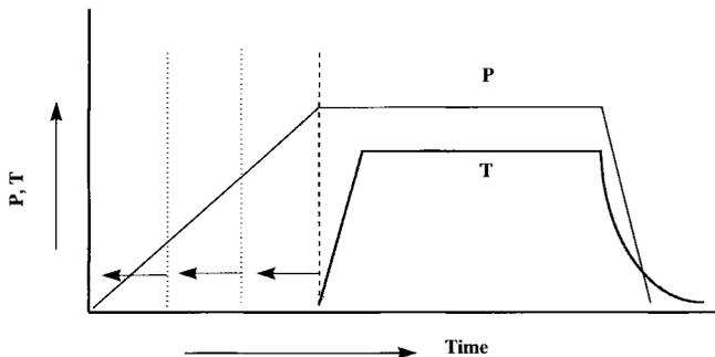
Fig. 8. Virtual experiment design for process optimization. The time-sequence of pressure ( $P$ ) and temperature ( $T$ ) ramps is schematically represented for a conventional process. Early heating is illustrated as advancing the heating initiation to positions indicated by the dotted lines.
