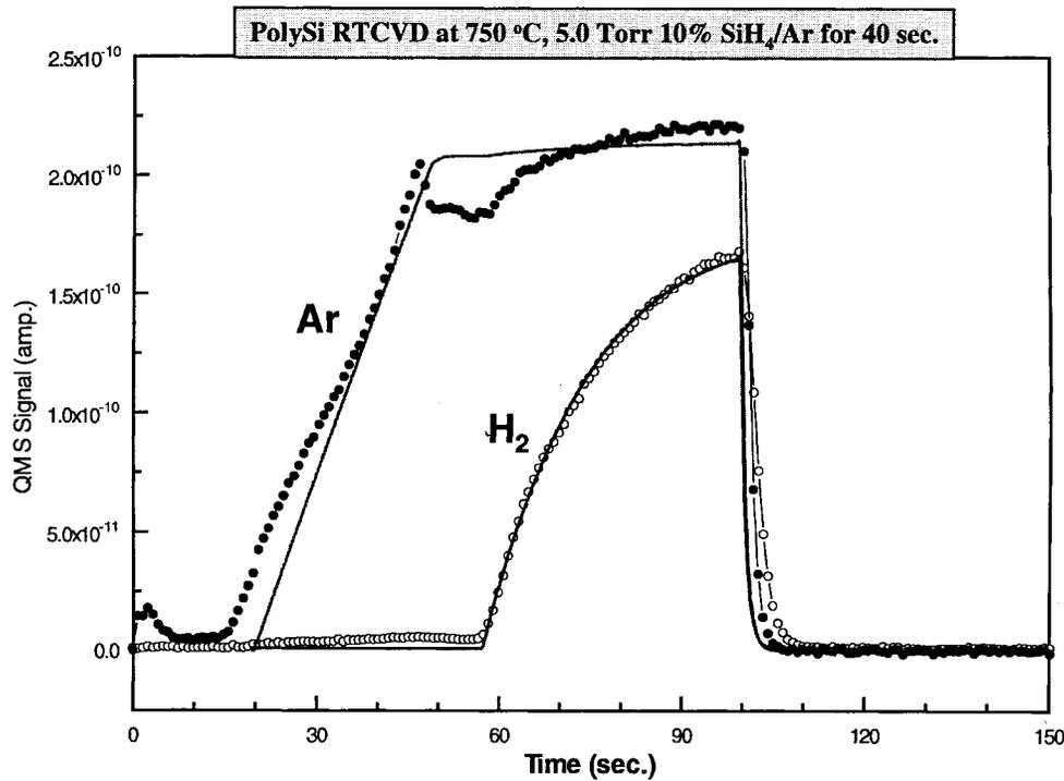
Fig. 5. QMS signals (ion current) for Ar and  $H_2$  throughout the whole process cycle for polysilicon RTCVD at  $750^\circ\text{C}$  and 5.0 Torr 10%  $\text{SiH}_4/\text{Ar}$  for 40 s. The circle data points are from actual experimental measurements, and the solid lines are from simulation.
